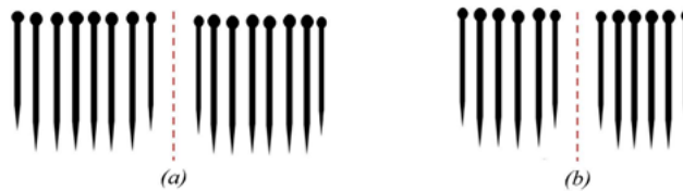
Figure 10. The pegs used to clamp the outrigger; a) 8 Pegs on the outside left and right bow with a total of 16 pegs; and b) 6 Pegs on the outsidebow left and right, with a total of 12 pegs.
